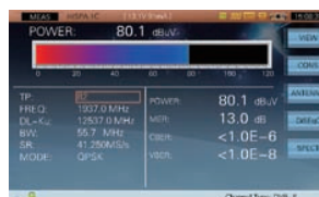
DVB-S/S2 Signal Measurement
