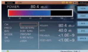
QAM signal quality measurement
