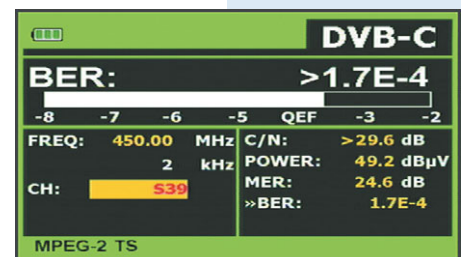
Digital cable (DVB-C) measurements
