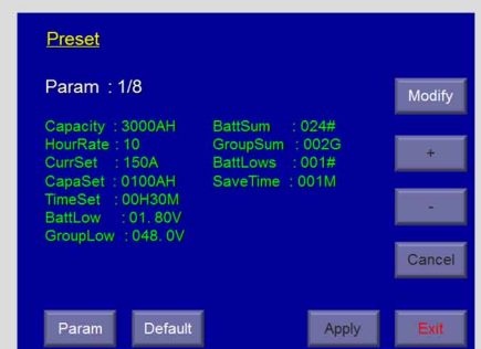
Presetting function speed up the setting
