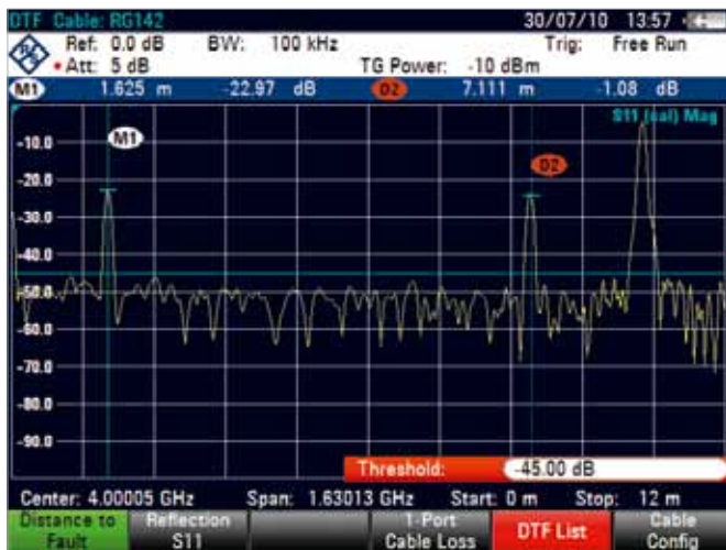
Distance-to-fault (DTF) measurement.
