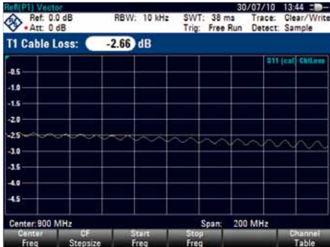
One-port cable loss measurement.
