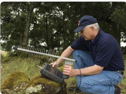
Locate interference signals
