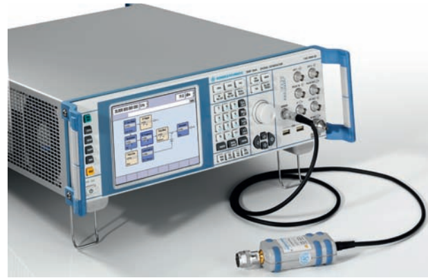
An R&S®NRP-Zx power sensor attached at the sensor connector
