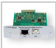
Ethernet/USB-Interface H0730 for industrial Use (Option)
