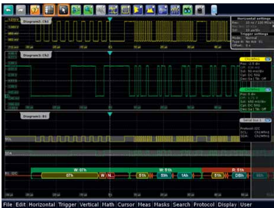
The high acquisition rates make it possible to find and display protocol errors quickly.
