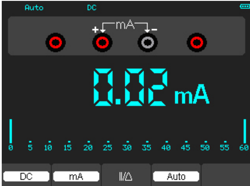
Figure 4-8 DC current Measurement for 600 mA
