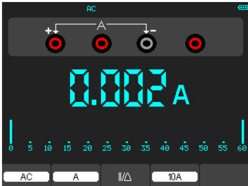
Figure 4-11 AC Current Measurement for 10A
