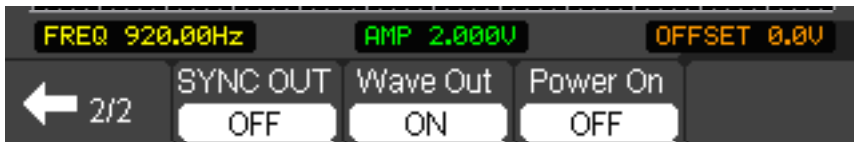
Figure 5-4 The Waveform Generator menu
