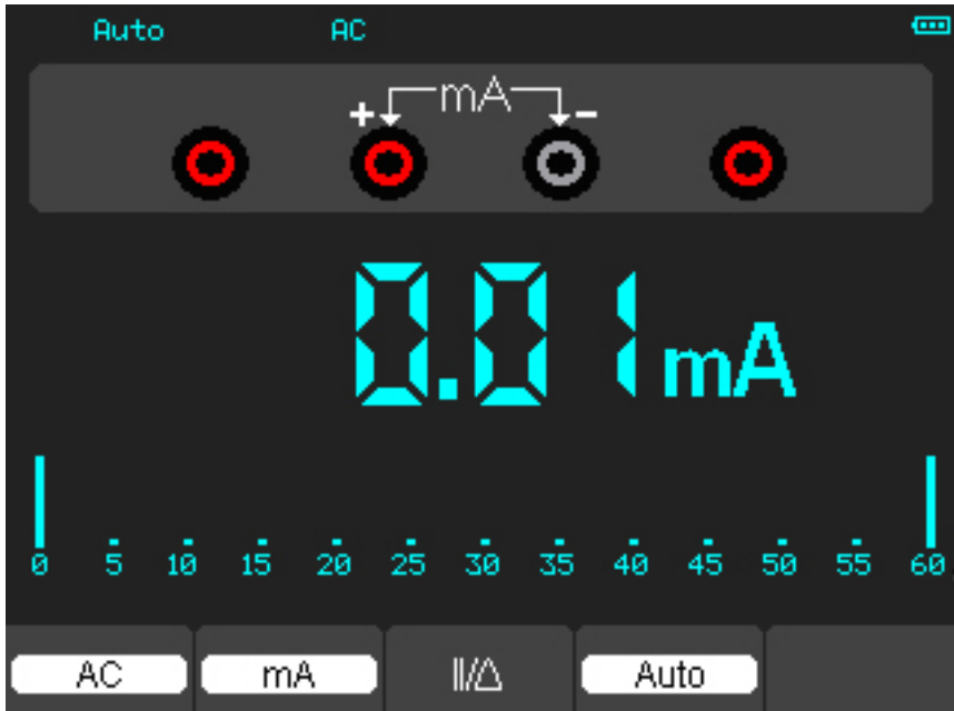
Figure 4-10 AC Current Measurement for 600 mA
