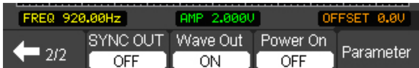
Figure 5-8 The Waveform Generator menu
