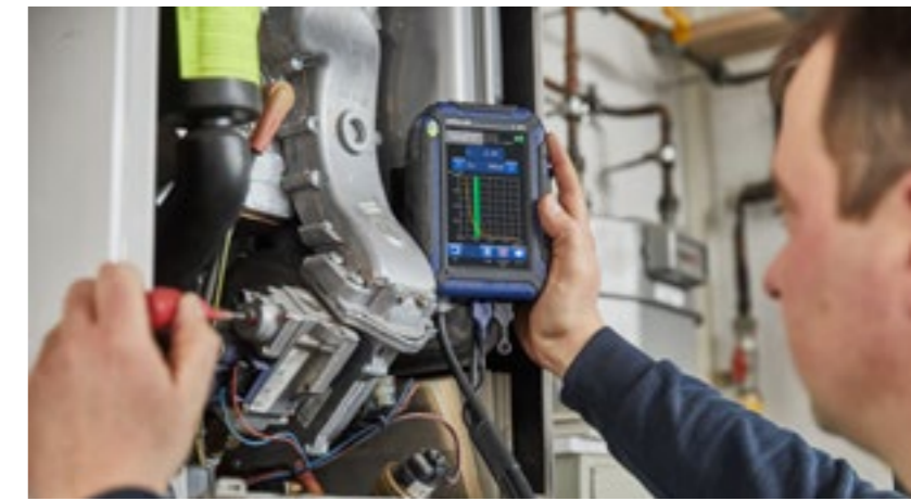
Tuning Guide: Graphic tuning guide for quick and reliable setting of the required value.
