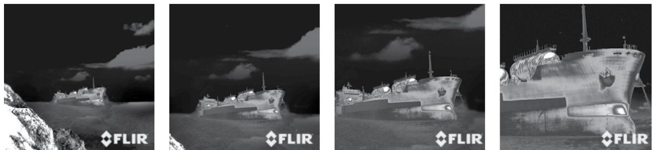
HRC-Series equipped with a continuous optical and continuous digital zoom on the thermal image allowing to have a closer look at objects which are far.
