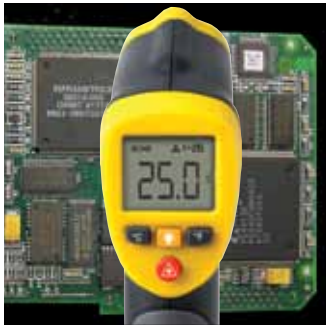
IR thermometer, measures temperature in one point
