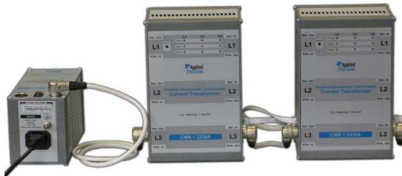
Power Supply PSCI 1220A connected to CMR-I units
