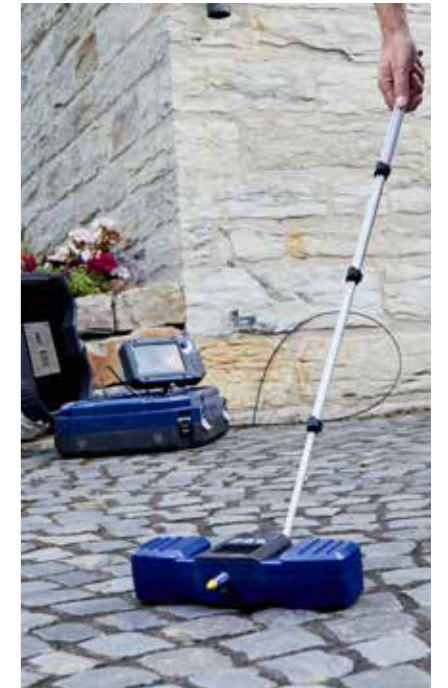
With the Wöhler L 200 Locator, the camera head can be located with pinpoint accuracy.
