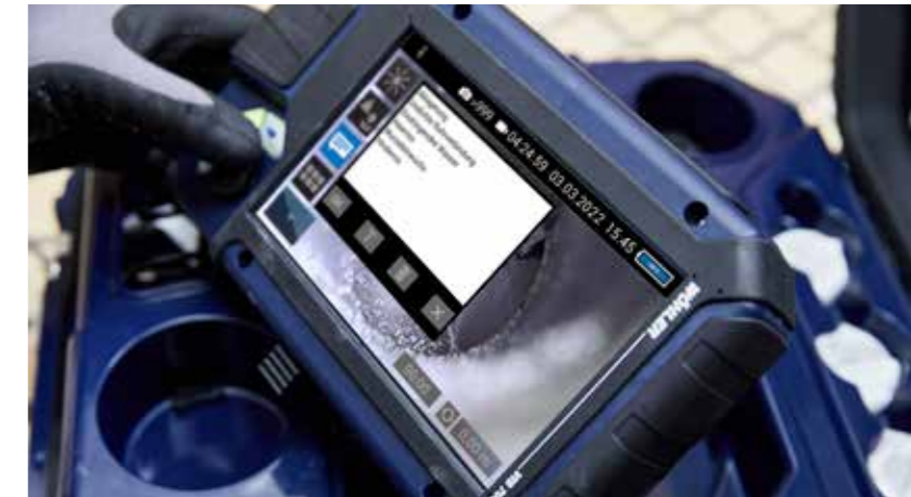
You can add your own or predefined commentary to each image. Voice comments on video recordings are also possible.
