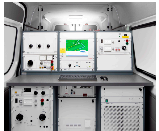
Installation in cable test vans
