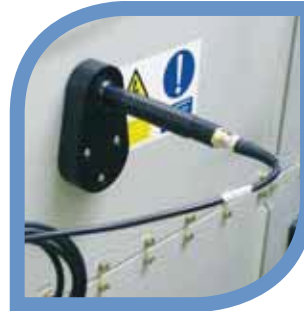
Options include (from top left): ultrasonic microphone, contact ultrasonic sensor and plug-in TEV probe
