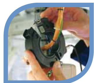
PD activity in cables is monitored using Radio Frequency Current Transformer (RFCT)
