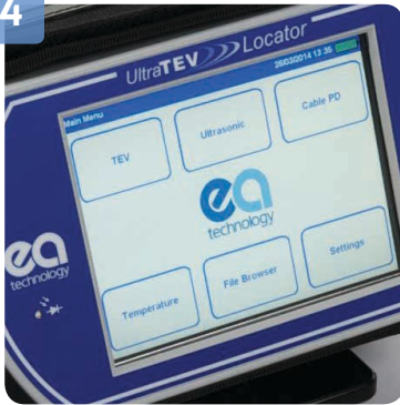
Simple touch-screen navigation between functions, including browser for stored data files
