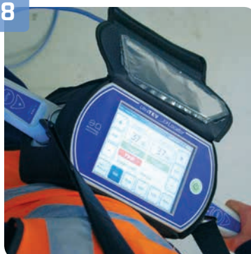
Integral Function Checker confirms the instrument is operating correctly
