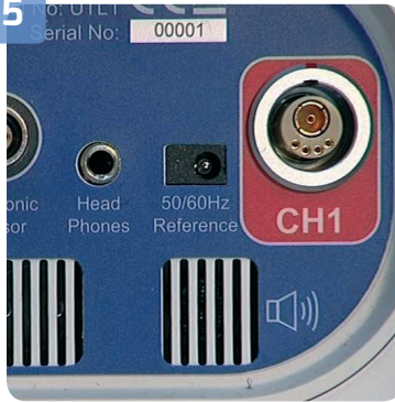
A phase reference is used to synchronise PD with the local power frequency, this is provided by either a plug in phase reference supplied with the instrument or optically from any nearby mains powered lighting source
