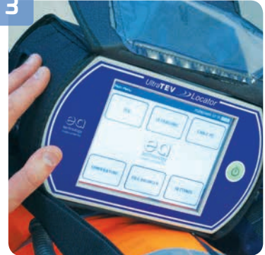
High resolution touch-screen - can be operated through the carry case cover
