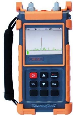
OFI-50A uses optical fiber sensing principle to confirm the target fiber; It can quickly identify deep buried, overhead and pipe fiber cable without any destroy, and provide a simple method for maintenance personnel. Users only need gently knock on cable, when knocking to the target cable, OFI-50 can clearly hear the knock from earphone, which can accurately identify the target cable.
