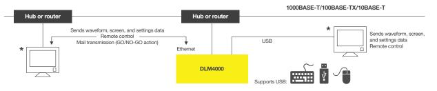
\*DLM4000's internal storage can be recognized by a PC as an external USB storage device. Transferring files is easy even when a USB thumb drive can't be used.
