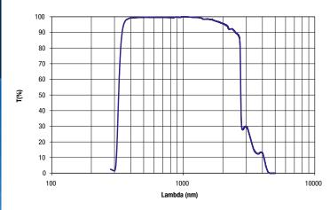
Graphic 1: Relative spectral response of the Delta Ohm pyranometers.
