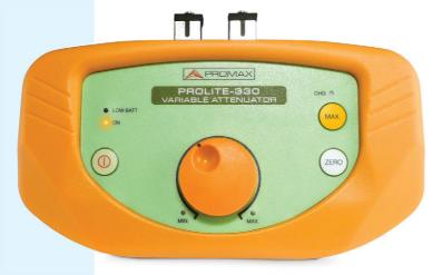
The **PROLITE-330** is a variable optical attenuator delivering more than 30 dB. It is a very low cost instrument designed for general use in R+D labs as well as field applications when a variable attenuation of signal is required. You can know exactly the chosen attenuation in combination with a power meter. Specially designed for FTTH networks and devices.
