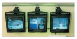
TDK RF Solutions' EUT Monitoring System integrates monitoring instrumentation, video and audio equipment, and software to provide EUT signal monitoring, EUT stimulation, and monitoring for visual or audio interference during testing.
