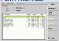
Saves and manages measurement trace and its state in the internal memory
