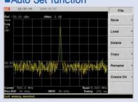
Automatically displays and sets maximum signal trace
